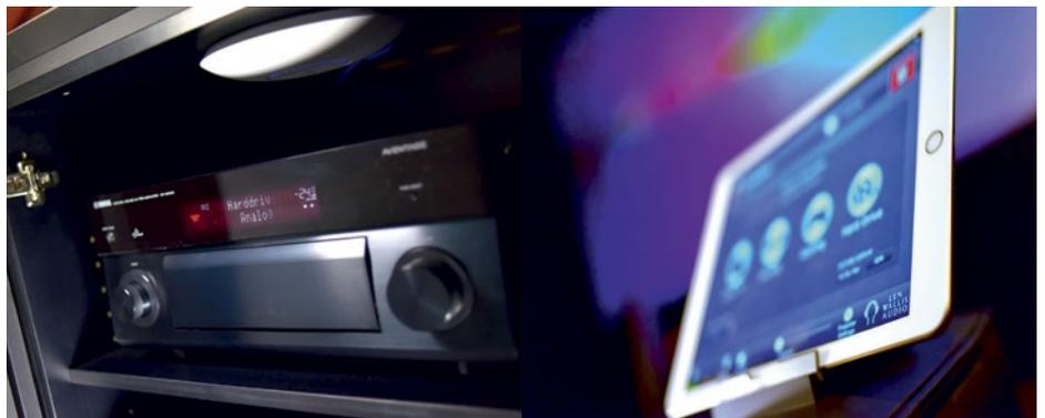
seat we provided them with an all-in-one iPad touch screen running the RTI control system. Once programmed the room could be used with the simplest of ease, with minimal button presses, seamless reliability and control, with macro functions programmed to speed and simplify operations still further. For example pressing the 'Blu-ray' icon turns on the Yamaha Pre and Power, switches to the correct input on the Yamaha, turns the projector on and selects its correct input, too – leaving the owners
